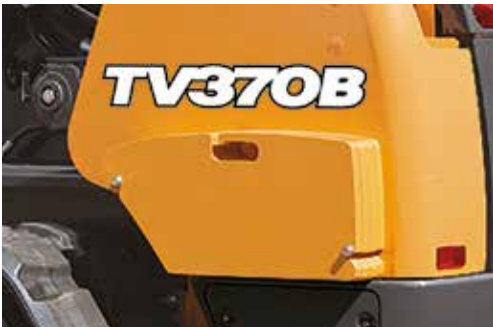
Additional Counterweight to increase ROC
