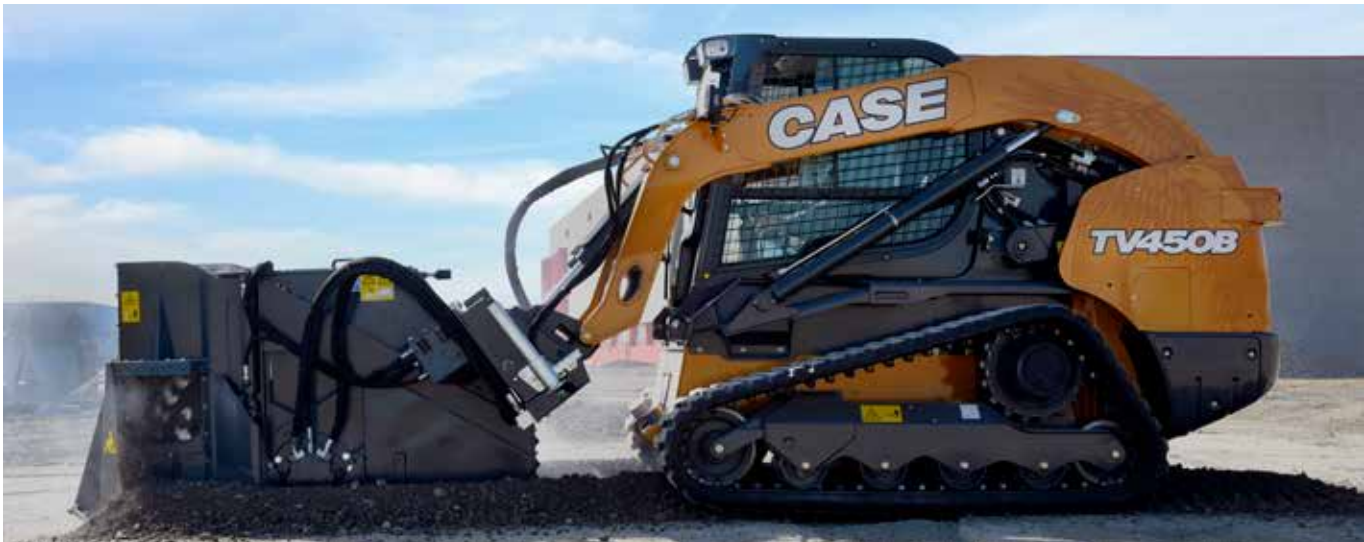
Additional Counterweight to increase ROC
