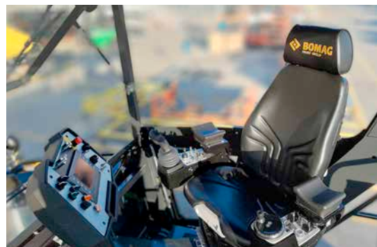
The right position in any situation – the comfortable driver's cab with swivel seat concept.
